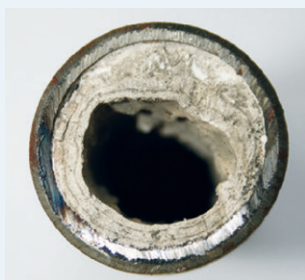
Example of calcium carbonate scaling
