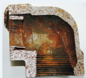
Example of corrosion inside a pipeline
